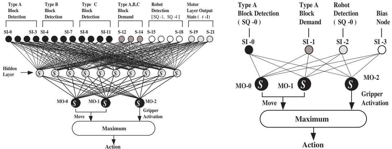
Fig. 3. *CONE-2 (Left) NEAT (Right) Controllers.* NEAT initializes a homogenous controller population subject to *complexification*. The NEAT controller illustrated is an example only. Controllers are initially random sensory-motor configurations (right). *CONE-2* uses a controller with a fixed topology (left).
