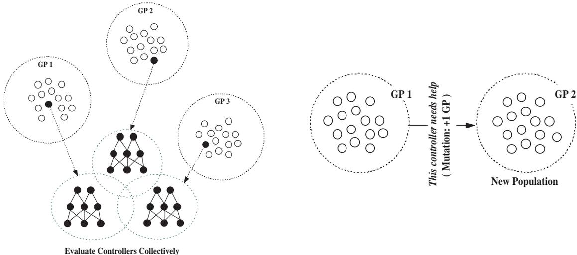
Fig. 1. *CONE-2 Example (Left)*: Three ANN controllers are derived from three *Genotype Populations* (GP) and evaluated collectively. Recombination only occurs *within* populations. *Team Size Adaptation (Right)*: Adding a genotype (controller) population (GP) and thus a new robot to the environment.
