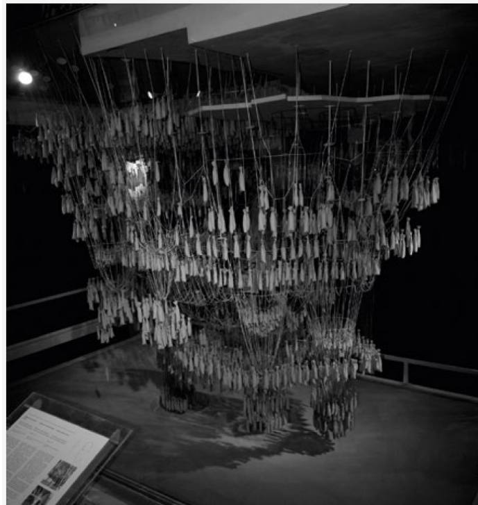
Figure 11: 1:15 scale reconstruction of Gaudí’s hanging model (Burry)
