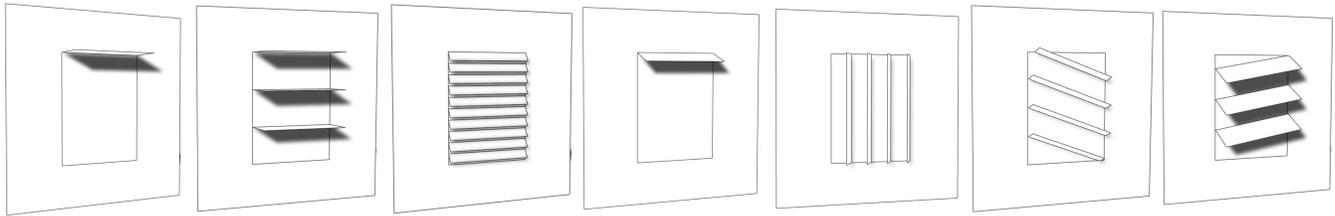
**Figure 1: From far-left: Traditional heuristically designed window sunshades: Horizontal overhang, overhang with three louvers, sloped 10 fins, steeper sloped overhang, vertical louver with four fins. Inner-right: Example evolved sunshade (Cape Town) from final NSGA-II Pareto front, with upward-angled fins to admit winter sun. Far-right: Example sunshade (Nairobi) from final MO-CMA-ES Pareto front, featuring downward-angled fins to reduce solar heat gain.**
